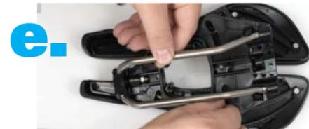
**e.** Replace the bolts and washers. Use the longest set in the back and the mid length set on the front. Your shortest set will be left over when using wedges. Adjust as needed. MAX torque 25 in/lbs or 2.8 NM
