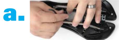
**a.** To install the wedges, remove the four bolts from the bottom of the saddle. NOTE: The REAR bolts are slightly longer than the front bolts.
