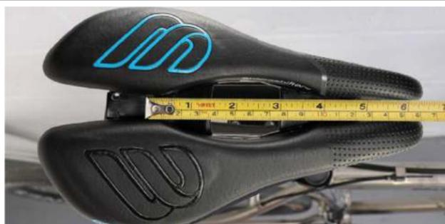
To set the height, simply replicate the height you measured on your old saddle. You may also want to adjust the tilt of the saddle top. We suggest starting with the top of the saddle flat, or slightly tilted downwards.
