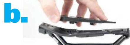
**b.** Place the wedge on the saddle frame, ensuring that it is properly aligned. Press down so alignment knobs can engage frame.
