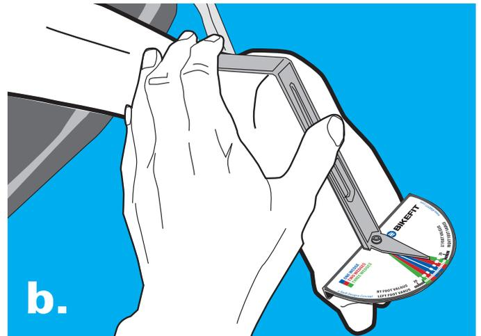
**b.** Place the Forefoot Measuring Device (FFMD) on the bottom of each foot pushing the handle against the heel so the vertical portion is aligned dividing the heel in two equal halves.
